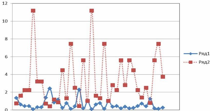
Figure 4 – Relationship between differentiation eutectic colony (line 1) and local rate of crystallization (line 2)
