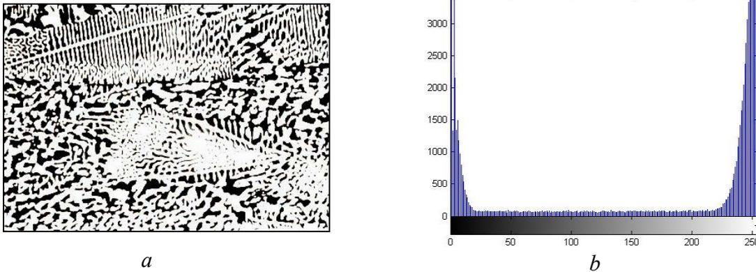
Figure 2 – Alloy Fe-B: photography x500 (*a*); color histogram (*b*)
