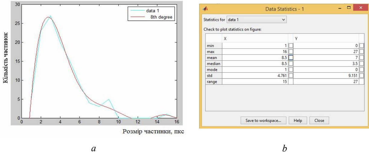
Figure 3 – Distribution of particles phase Fe<sub>2</sub>B in the alloy Fe-3,8% B of a size (a); statistics (b)
